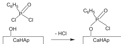
Scheme 1. Representation of the first step of the reaction between the phenyl phosphonic dichloride and the hydroxyl groups on the surface of the apatite, leading to covalent P–O–P bond with elimination of HCl.
